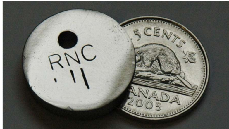
Ferronickel Button Produced Directly from Dumont Concentrate in Preliminary Testwork
